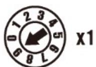
Each MODBUS Adapter could have an unique address (from 1 to 99) so that it can be addressed independently from other nodes.
