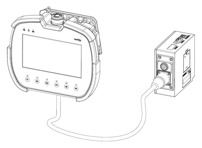
The cables to TOPRH0700WD can be made 3, 5, and 10M in length. (It is a twisted pair cable and should be properly wired for an intended purpose.)
