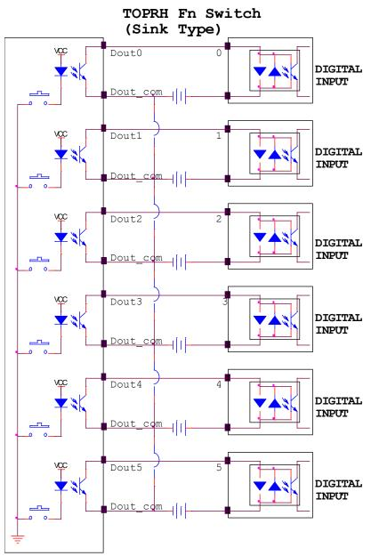
(\* It runs with a photocoupler, so it can be controlled only when the main body is on.)
