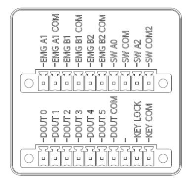
• Emergency switch: wiring diagram
