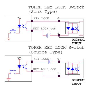
(\* It runs with a photocoupler, so it can be controlled only when the main body turns on.)
