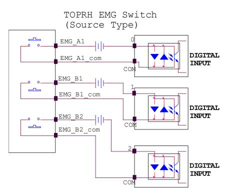
(\* It is a mechanical switch, which can operate regardless on/off status of main body.)
