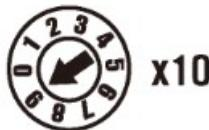
Node address set-up is rotary switch. Default Node Address is 1. Max node Address is 42.
