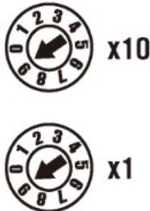
Each MODBUS Adapter could have an unique address (from 1 to 99) so that it can be addressed independently from other nodes.
