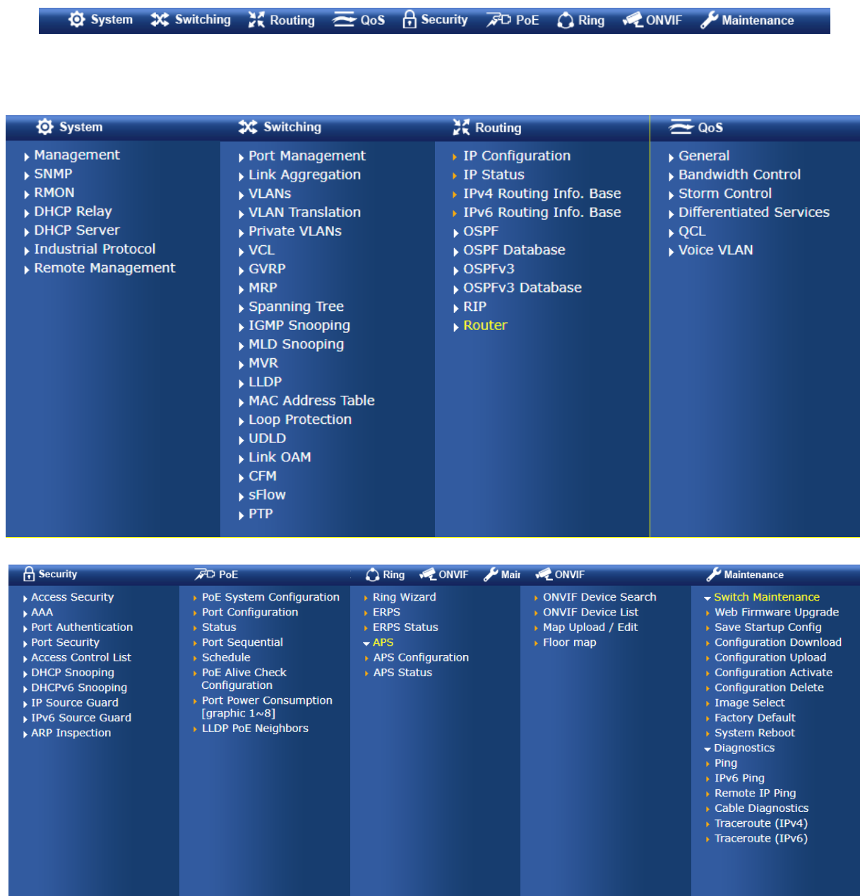
Figure 4-1-6: Managed Switch Main Functions Menu
