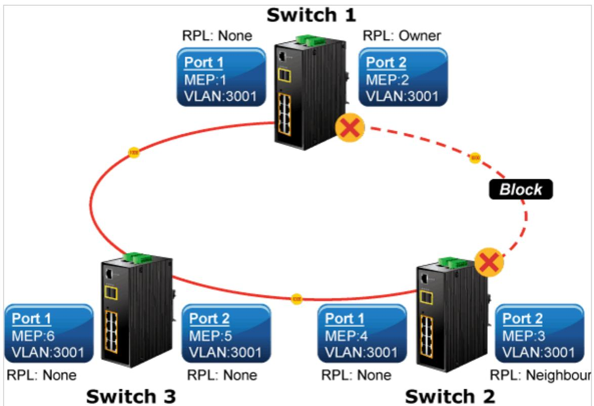
Figure 4-7-1-1: Ring Example Diagram
