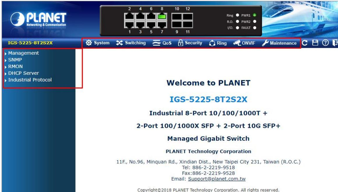
Figure 4-1-5: Industrial Managed Switch Main Functions Menu
