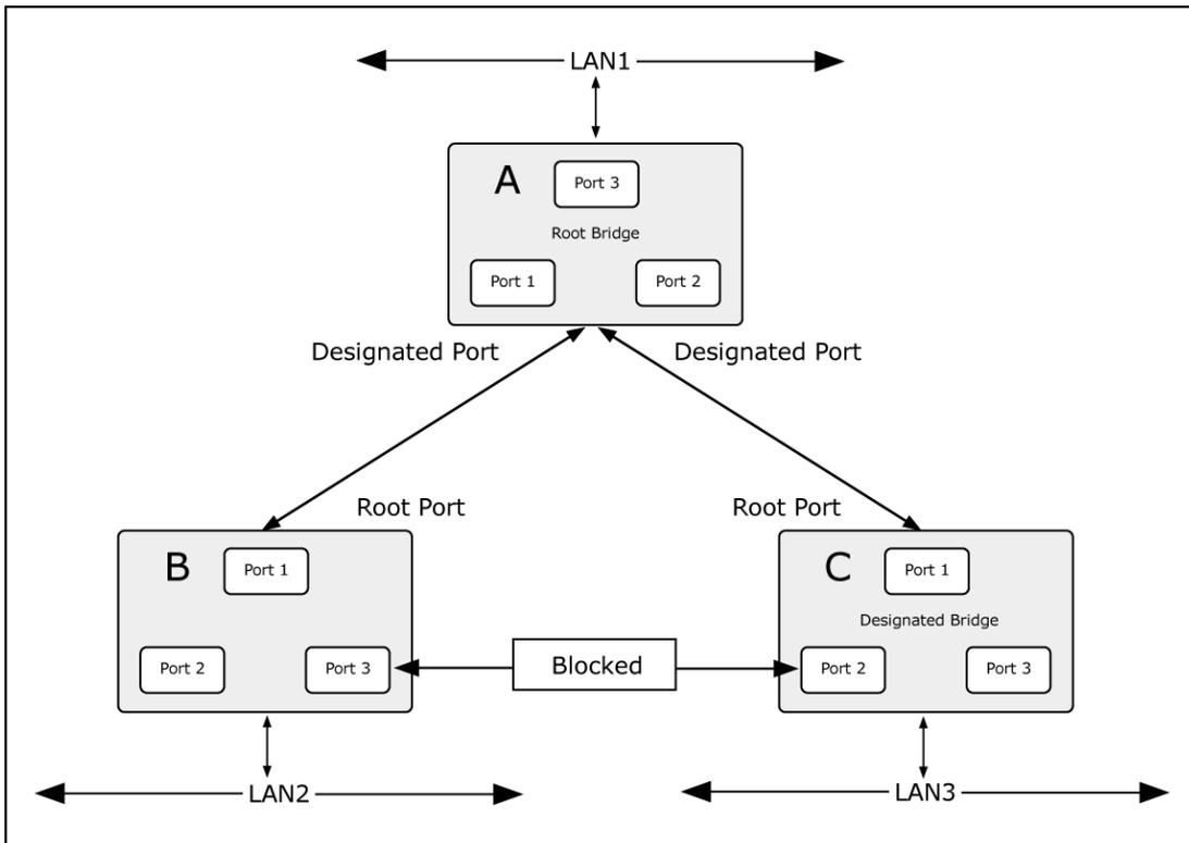
Figure 4-3-9-3: After Applying the STA Rules
