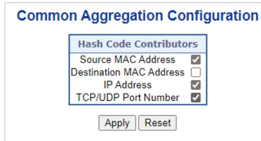
Figure 4-3-2-2 : Aggregation Mode Configuration Page Screenshot
