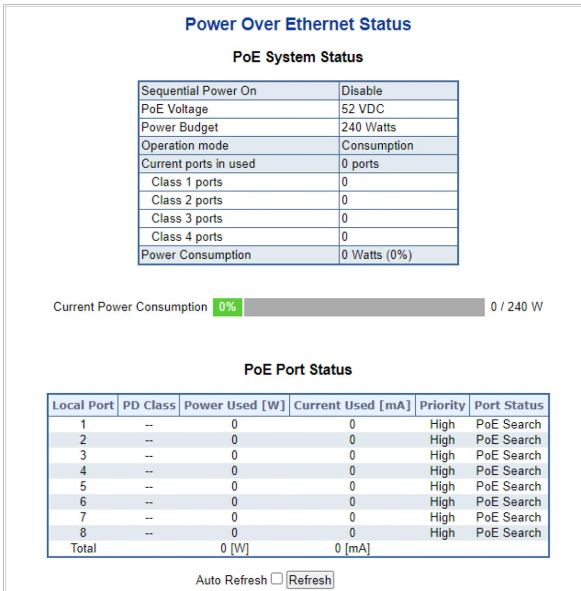
Figure 4-6-1-1: Power over Ethernet Status
