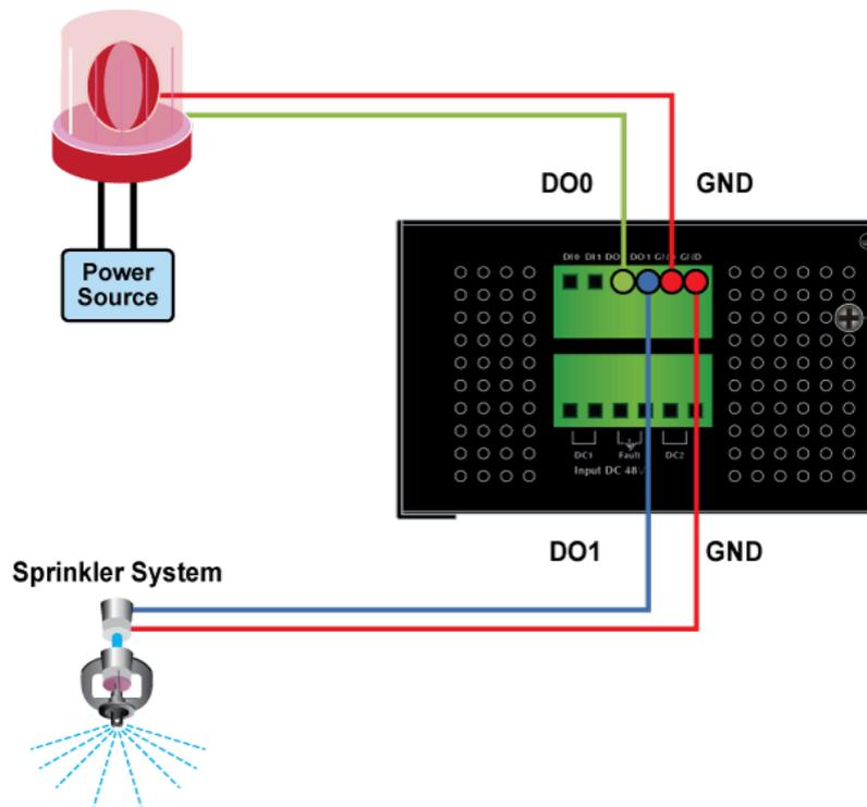
Figure 2-10: Wires DO0 and DO1 to Open Detector
