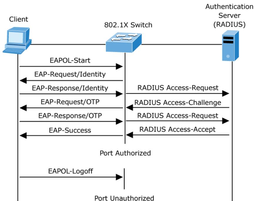
Figure 4-5-2-2: EAP Message Exchange
