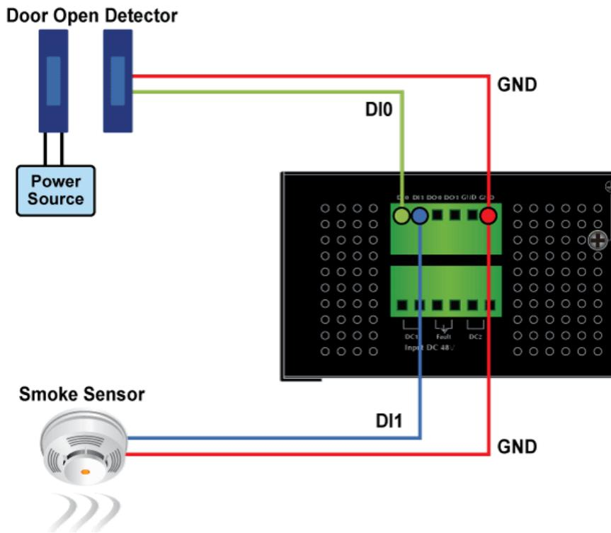
Figure 2-9: Wires DI0 and DI1 to Open Detector
