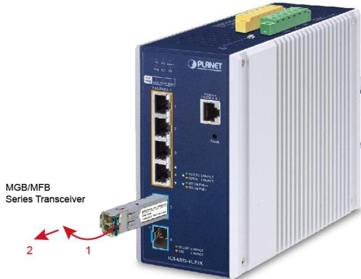
**Figure 2-12:** Pull out the SFP/SFP+ Transceiver Module
