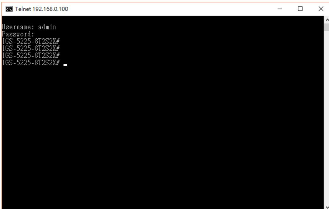
Figure 3-4: Remote Telnet Interface Main Screen of Industrial Managed Switch
