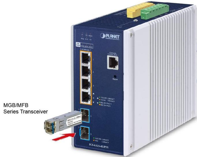
**Figure 2-11:** Plug in the SFP/SFP+ Transceiver
