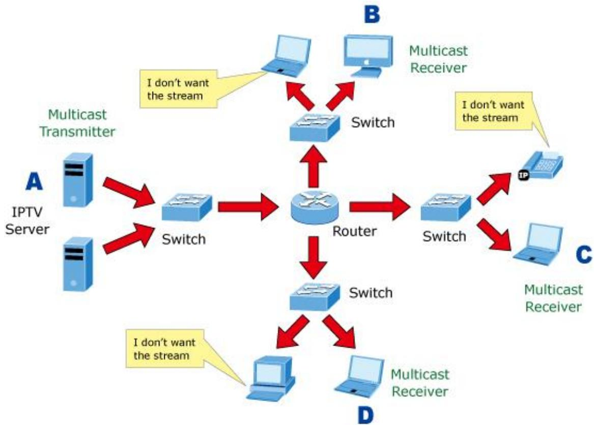
Figure 4-3-10-2: Multicast Flooding
