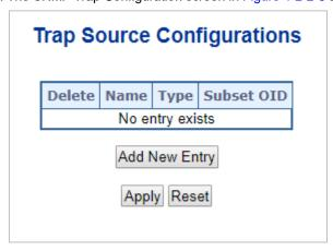
Figure 4-2-2-5: SNMP Trap Source Configuration Page Screenshot
