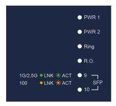
Figure 2-1-2: LED Panel of WGS-5225-8UP2SV
