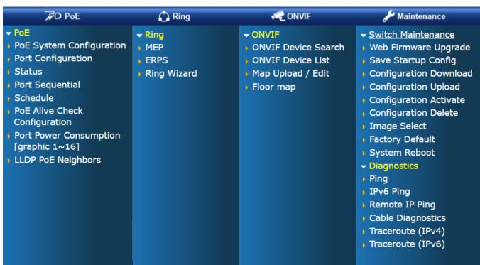
Figure 4-1-5: Managed Switch Main Functions Menu
