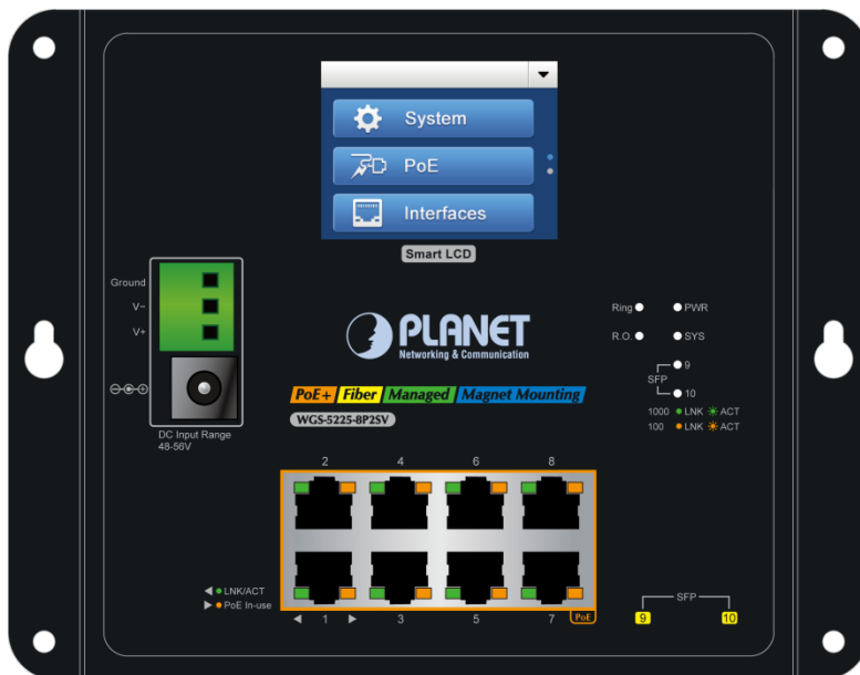
Figure 2-1-1: Front Panel of WGS-5225-8P2SV
