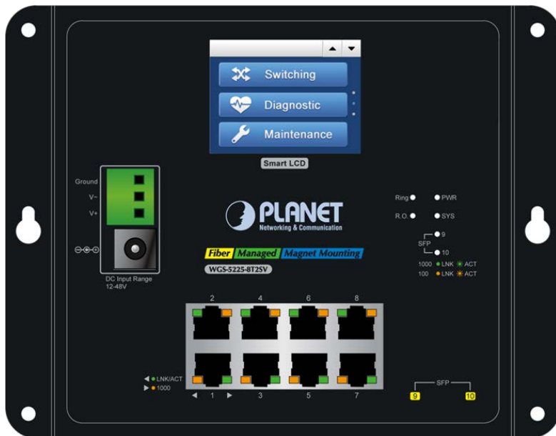
Figure 2-1-3: Front Panel of WGS-5225-8T2SV
