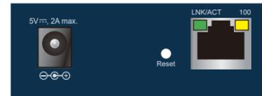
Figure 3-1: Rear Panel of MG-120.
